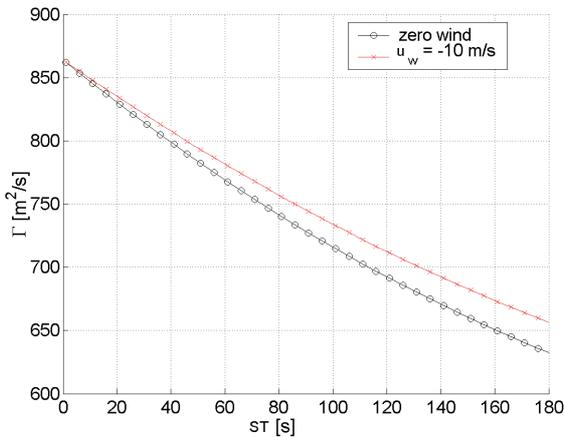
**Fig. 10 Circulation over separation time for zero wind and  $u_W = -10$  m/s at  $x_{gate} = -11$  nm from runway threshold**
