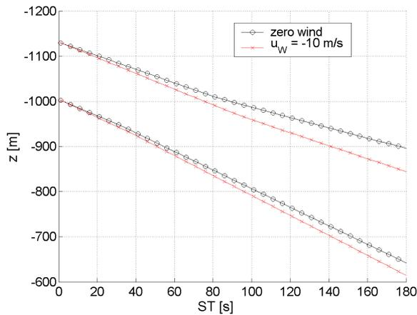
**Fig. 11 Vortex height over separation time for zero wind and  $u_W = -10$  m/s at  $x_{\text{gate}} = -11$  nm from runway threshold**
