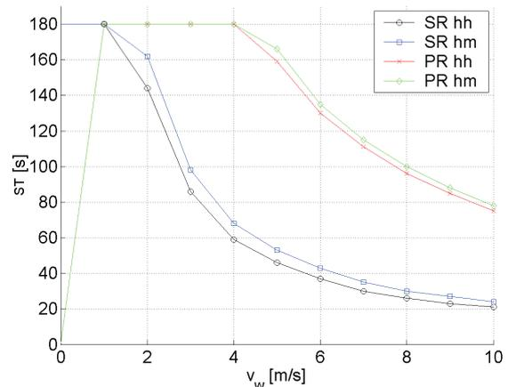
**Fig. 5** Comparison of separation times for different A/C classes (met 1,  $RCR_{nom} = 20\%$ )
