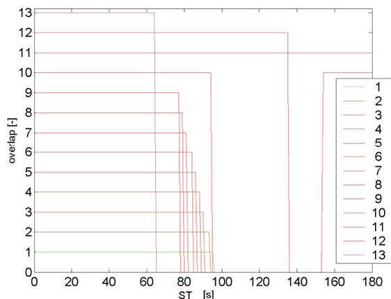
**Fig. 12 Overlapping of approach corridor and overall hazard area for gates along the glide path for headwind  $u_W = -10$  m/s**
