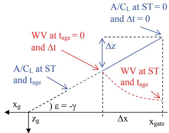
**Fig. 8 Approach situation with headwind**
