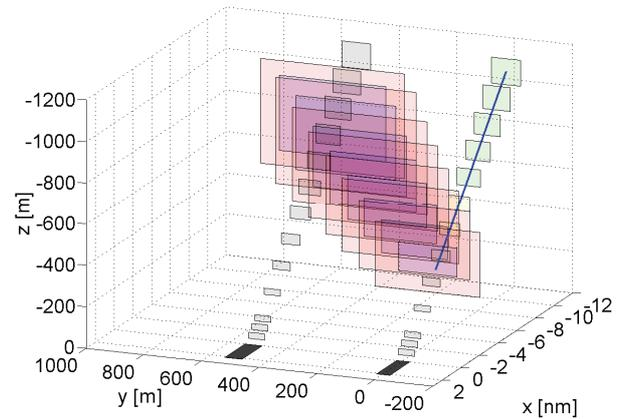
**Fig. 4** Parallel runway scenario with wake vortex habitation area and overall hazard area for cross wind  $v_w = 3$  m/s (hm, met 2,  $RCR_{nom} = 20\%$ )
