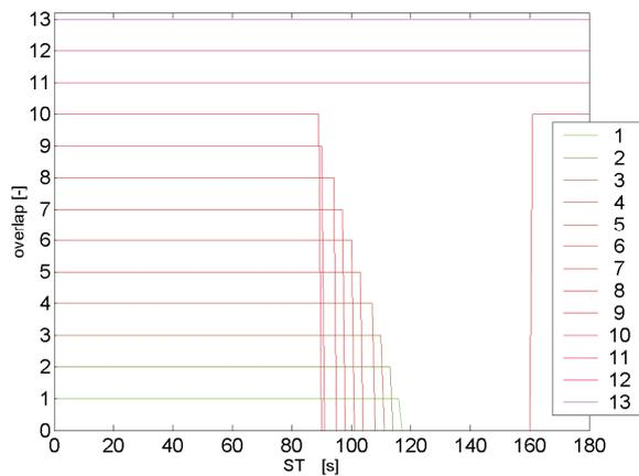
**Fig. 3** Overlapping of approach corridor and overall hazard area for gates along the glide path for calm air
