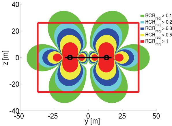
**Fig. 1 Wake vortex induced required roll control power and simplified hazard area (SHA, for  $RCR_{nom} = 20\%$ ,  $t_{age} = 50$  s, example ICAO pairing 'light' behind 'medium', no turbulence) in the cross section behind the vortex generating aircraft (with indicated generator wing and vortex cores)**
