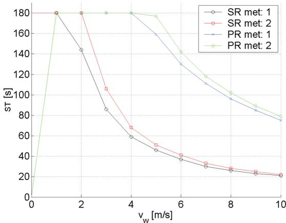
**Fig. 6 Comparison of separation times for different meteorological conditions (hh,  $RCR_{nom} = 20\%$ )**
