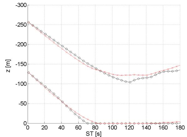
**Fig. 13 Vortex height over separation time for zero wind and  $u_W = -10$  m/s at  $x_{\text{gate}} = -2$  nm from runway threshold (gate 10)**
